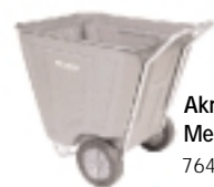
Wheels and Axles: Medium-duty 60 and 90 gal. Akro-Carts feature 12" dia. wheels, high-impact plastic hubs with semi-pneumatic tires and 16-gauge steel tubing axle.
