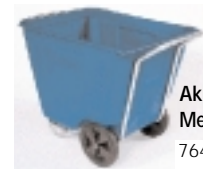
Wheels and Axles: Medium-duty 60 and 90 gal. Akro-Carts feature 12" dia. wheels, high-impact plastic hubs with semi-pneumatic tires and 16-gauge steel tubing axle.
